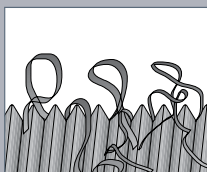
Poor Chip Control
