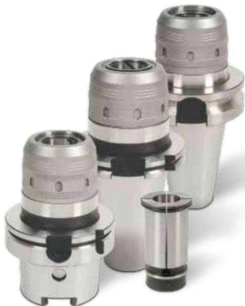
The high gripping force achieved by the **MAXIN POWER CHUCK** results from the shallow nose tapered cone (1) with helical slot (3) inside the internal chuck bore. It exerts a very high clamping force when the clamping nut (2) is rotated in the axial direction. The shallow taper of the tool nose (1) and the angled position of the needle bearing (4) that sit in the cage create the axial movement of the clamping nut (2).
