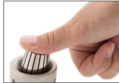
**Important:** Never insert the collet parallel to the extractor ring. Doing this will chip or break the extractor's teeth. When unclamping the nut, the collet will self-release from the chuck by means of extractor teeth.
